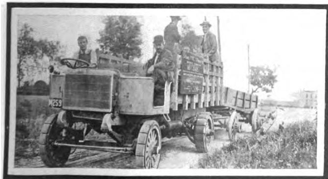
American-La France truck and trailer, hauling a load of 11 tons of bricks over a Jersey hill at 5 miles an hour
